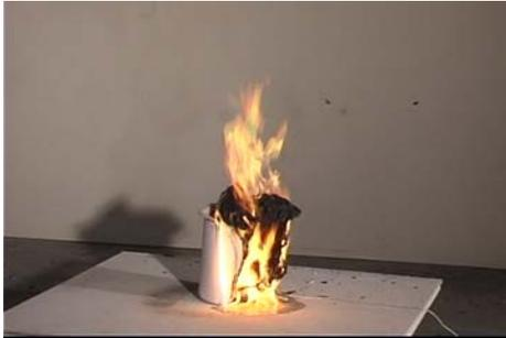
**Figure 3.2-3. Trash container 1, 200 s after ignition**
