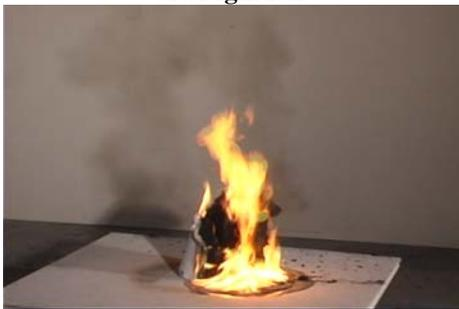
**Figure 3.2-5. Trash container 1, 400 s after ignition**
