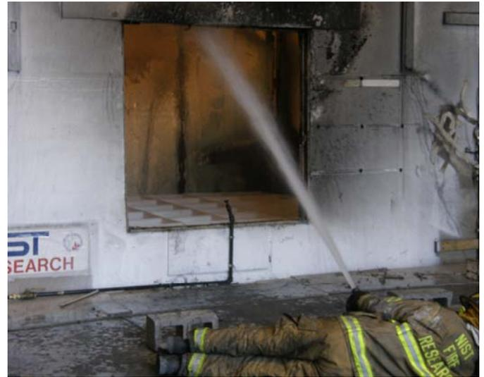
**Figure 4.3.3-4. Solid stream discharged into window opening.**
