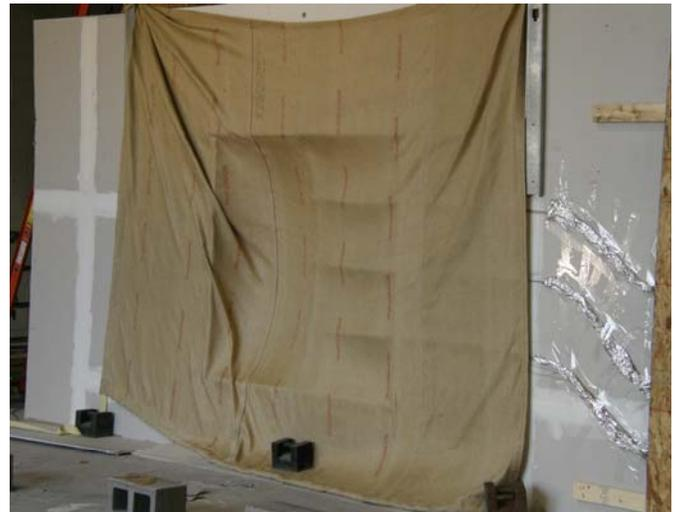
Figure 4.3.2-2. Large WCD deployed over window opening.
