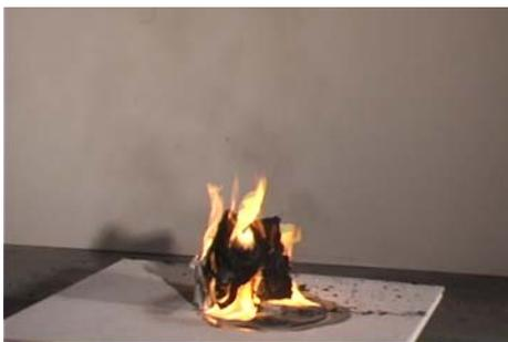
**Figure 3.2-7. Trash container 1, 500 s after ignition**
