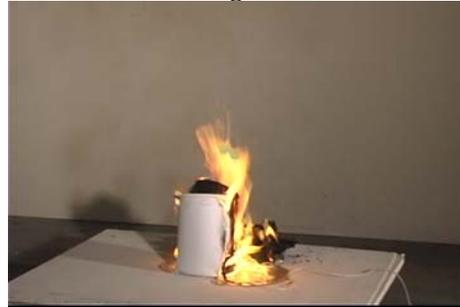
**Figure 3.2-12. Trash container 2, 300 s after ignition**
