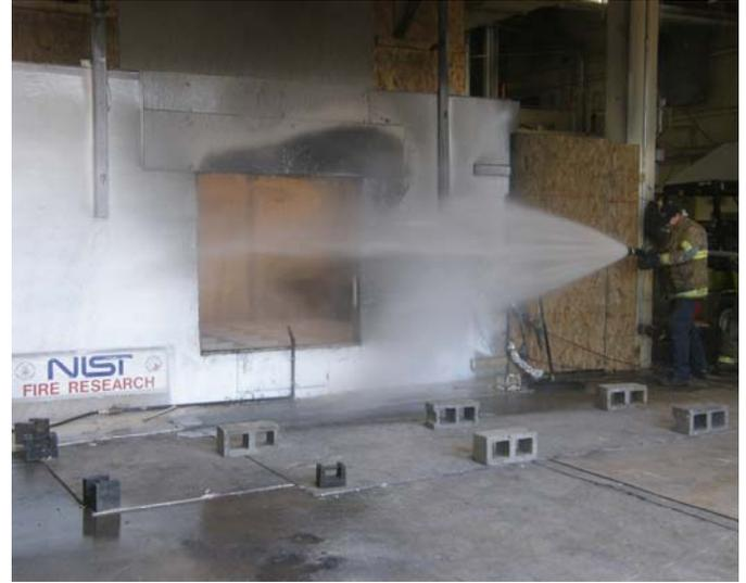
**Figure 4.3.3-2. Fog stream discharged across window opening.**
