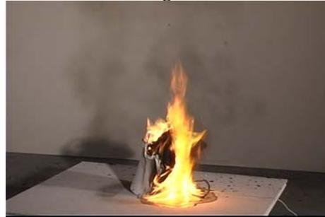
**Figure 3.2-4. Trash container 1, 300 s after ignition**
