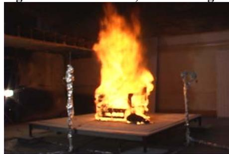
Figure 3.4.2-6. Chair 2, at peak heat release rate, 437 s after ignition
