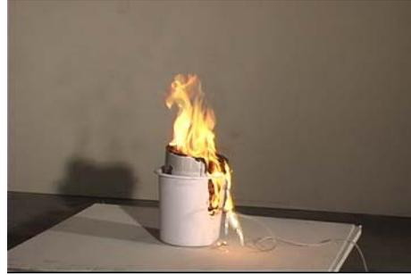
**Figure 3.2-10. Trash container 2, 100 s after ignition**
