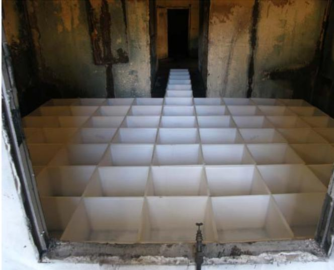
**Figure 4.3.3-1. Water spray distribution experiment arrangement.**
