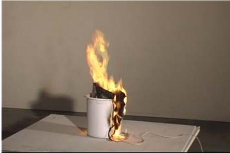
**Figure 3.2-11. Trash container 2, 200 s after ignition**
