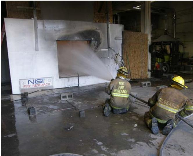
**Figure 4.3.3-3. Fog stream discharged into window opening.**
