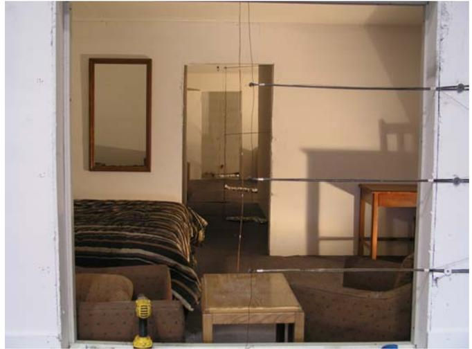
**Figure 4.1.3-3. Bi-directional probe array in west window.**
