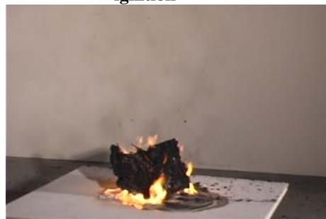
**Figure 3.2-8. Trash container 1, 600 s after ignition**
