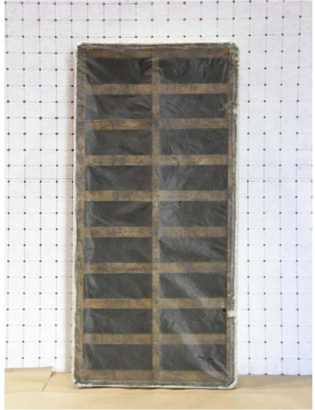
**Figure 3.3-2. Bottom side of box spring.**
