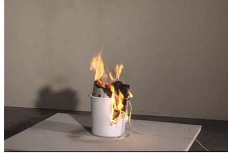
**Figure 3.2-2. Trash container 1, 100 s after ignition**
