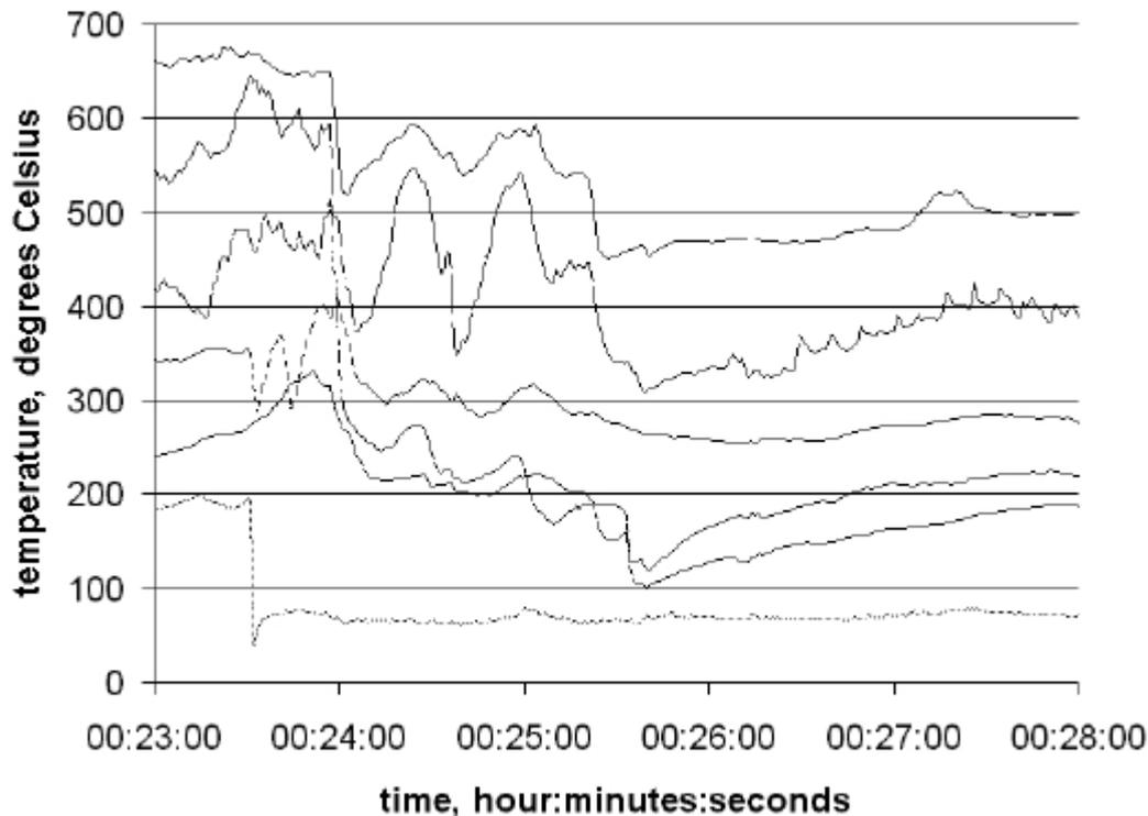
Fig 4 - 340LPM standard 38mm lay-flat attack hose-line demonstrating a 0.7mm mean droplet diameter during 'pulsing' application into the gaseous-phase using 0.5s - 2s pulses - failing to reduce the upper layer temperatures effectively (six temperature gradients recorded through the thermal layer). *Svensson & Sardqvist Report LUTVDG/TVBB-1025-SE Lund University Sweden 2002.*
