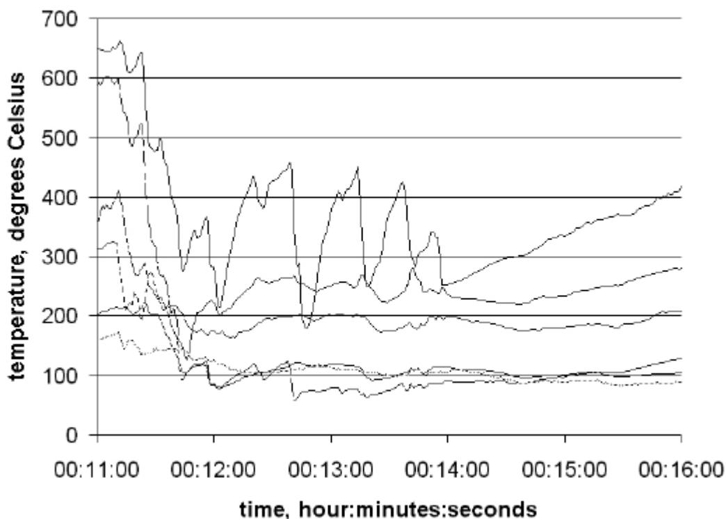
Fig 3 - 175LPM high-pressure 25mm hose-reel demonstrating a 0.2mm mean droplet diameter during ‘pulsing’ applications into the gaseous-phase using 0.5s - 2s pulses - reducing the upper layer temperatures by more than fifty percent through the evolution (six temperature gradients recorded through the thermal layer). *Svensson & Sardqvist Report LUTVDG/TVBB-1025-SE Lund University Sweden 2002.*
