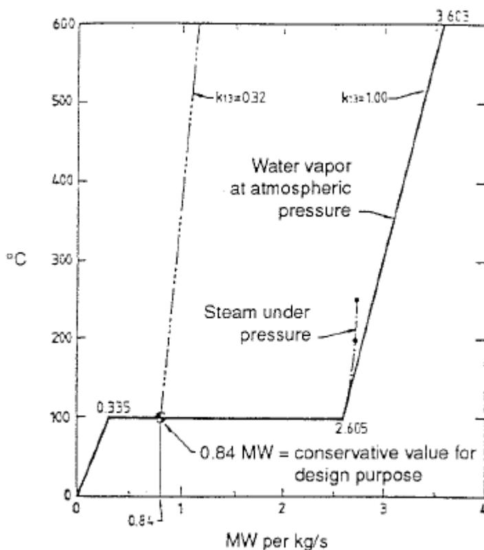
Figure 9 - Cooling power of water applied to a fire at the rate of 1 kg/s (1 litre/s)
