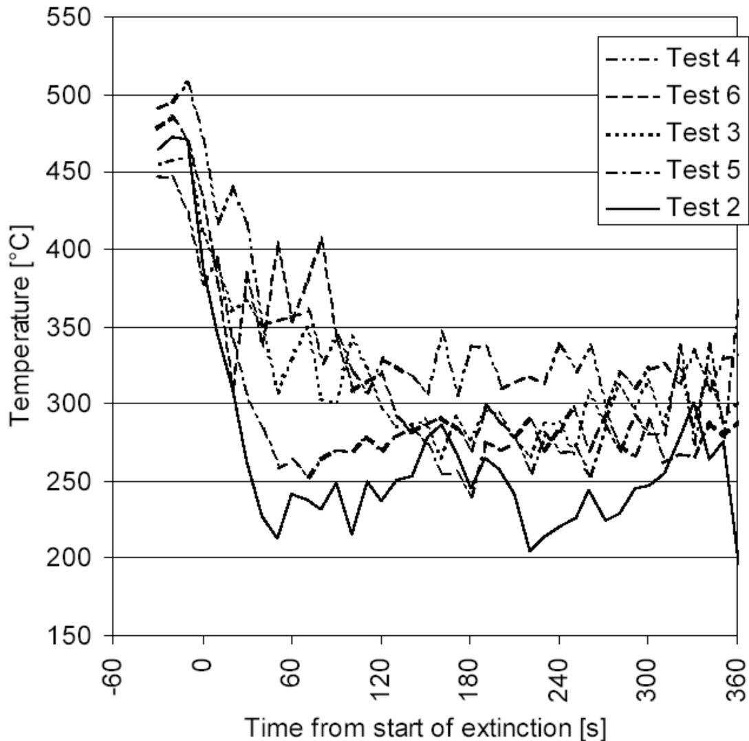
Figure 6 - The mean gas temperatures for all tests clearly demonstrate the greatest cooling effects were achieved during tests 2 & 5 (25mm high-pressure hose-reel) - although the flow-rate (113lpm) used in test 5 was unable to attain final control of the fuel-based fire within the test criteria of six minutes - Svensson & Sardqvist Report LUTVDG/TVBB-1025-SE Lund University Sweden 2002.
