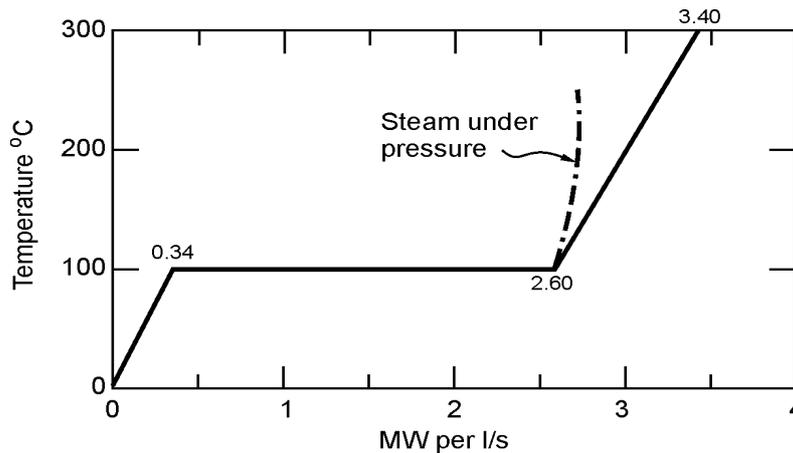
Figure 8 - Cooling power of water at 18°C applied to a fire at the rate of 1kg/s
