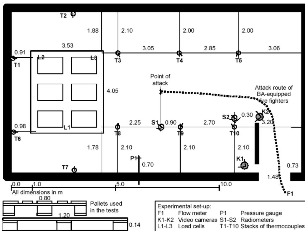
Figure 5 - The test set-up for the second series of tests in a 100m<sup>2</sup> compartment (Svensson & Sardqvist) - Svensson & Sardqvist Report LUTVDG/TVBB-1025-SE Lund University Sweden 2002.
