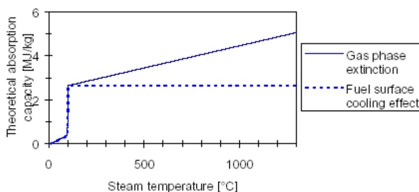
Fig 1 - Theoretical heat absorption capacity of water in the gaseous-phase and on surface cooling.
